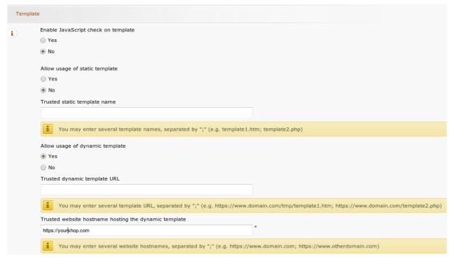
**Figure 2.1:** Configuration of the Dynamic Template.
