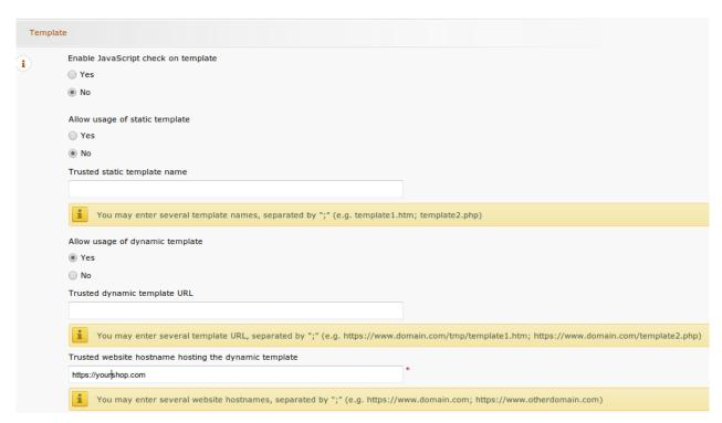
**Figure 2.1:** Configuration of the Dynamic Template.
